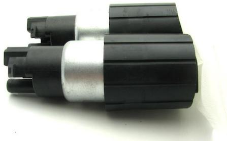
4 – install DW65c/300c pump and connect the hoses and electrical connectors
