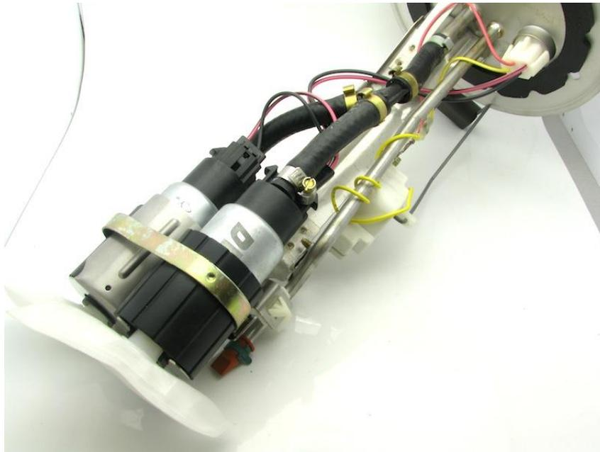
6 – reinstall the assembly into the fuel tank and attach a length of hose to the outlet of the pump assembly allowing it to drain into a fuel safe container and prime the fuel pump assembly
