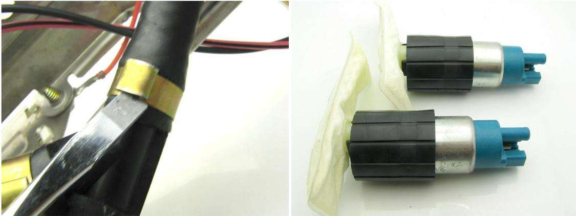
3 – reuse the pump isolators and install the fuel sock and sock retainer
