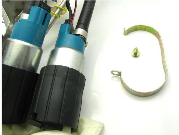
2 – loosen the OE hose clamps from both pumps and remove the pumps
