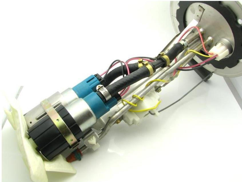
1 – remove the pump retaining strap
